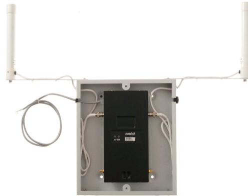
Antenna can mount on top or below enclosure.
